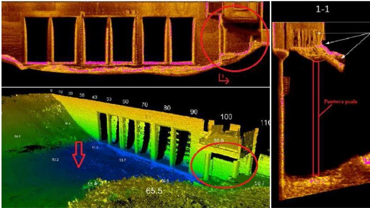
Figure 5. Comparison of details of 2D and 3D scans (case 3).
