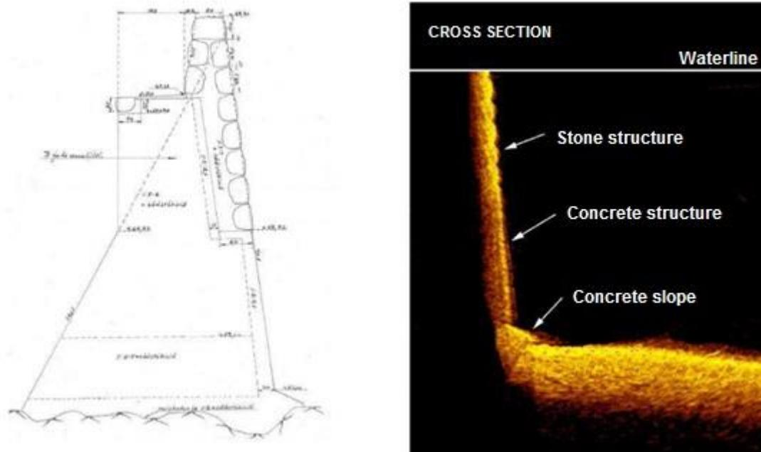
Figure 3. Sketches based on 2D sonar scan (case 2).
