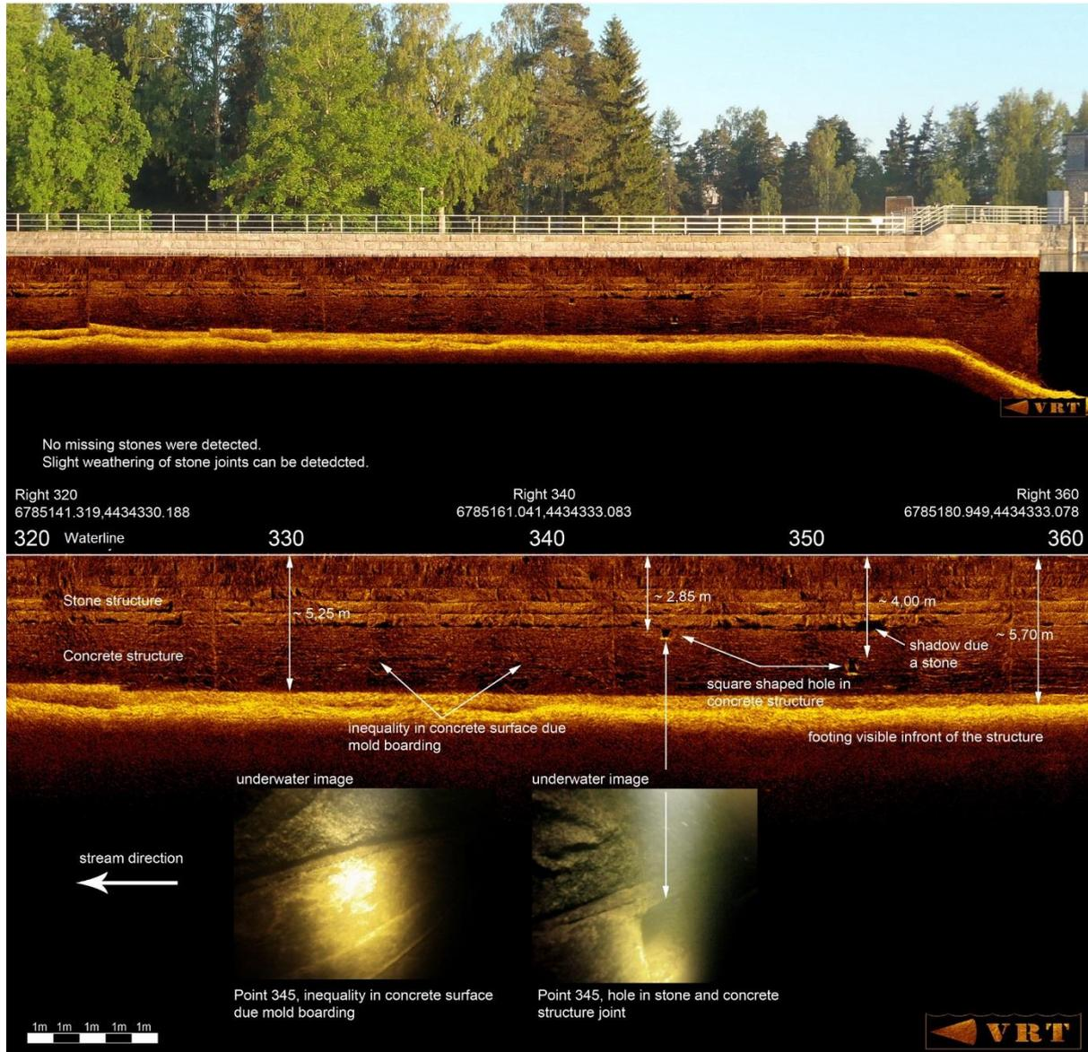
Figure 2. 2D Stationary sonar scan of vertical dam wall. Underwater pictures inset (case 2).
